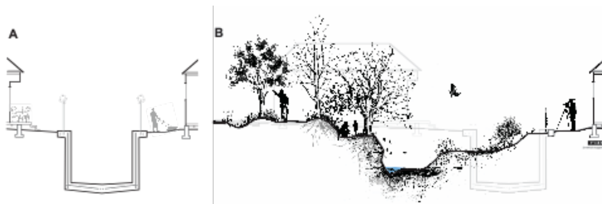
Figure 2-14. Comparison of idealized pre- and post-restoration cross sections for Grayson Creek. In A, the current concrete flood control channels have smooth, reinforced beds (to resist erosive flows) and vertical banks. Because flows are fast and dangerous, razor wire fences line the top of bank. Beyond this lie private properties and structures that require protection from floods. In B, an idealized restored cross section has free channel boundaries, vegetation, irregular form, gravel bars and pools, overhanging trees with potential to drop large branches, and more hospitable habitat for fish and wildlife. The increased roughness in B will slow in-stream flows and expand flow volumes. To prevent flooding of structures (i.e. on the right bank), the floodable area will need to widen considerably compared to A. The rougher the elements of the restored stream channel, the wider the floodable area will need to be.
